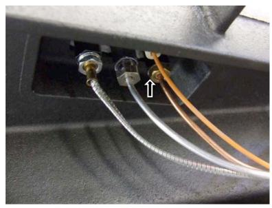
8. Pull the thermocouple down and out of the bracket.
